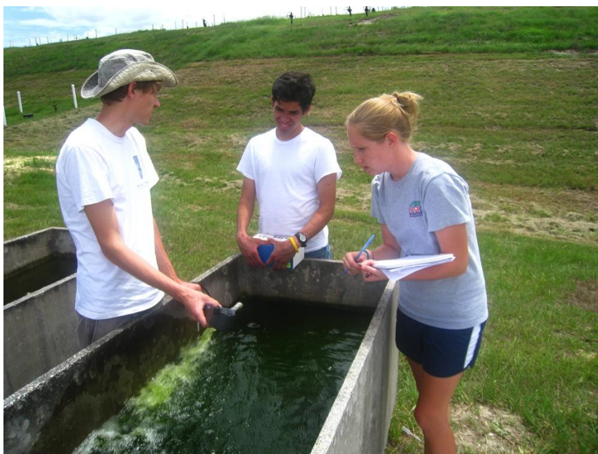
Figure 6. Algae growing in the 800L bioremediation tank on-site at the Alachua County South West Landfill. The closed municipal solid waste landfill is visible in the background.
